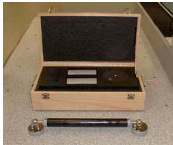
figure 4, Ball Bar Test Set
