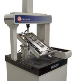
The U/V Rotary Table is manual in its operation and requires the operator to position the table to various positions. The supplied locks keep the table in position.
