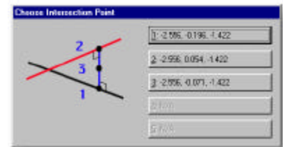
figure 5.8c, 3D Axis Intersect
