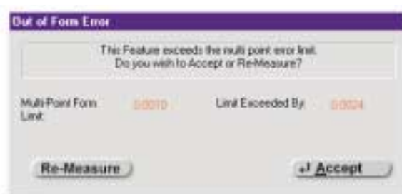
figure 4.4b, Form Error Limit
